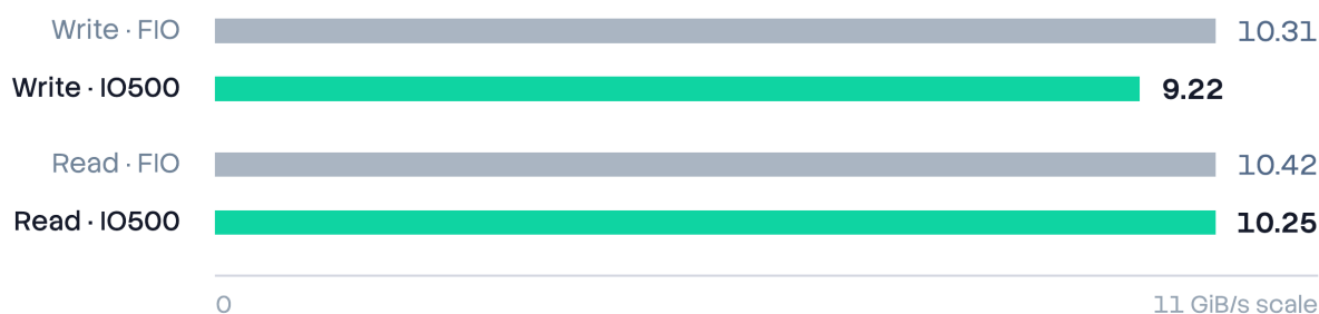
FIGURE 1 · SEQUENTIAL BANDWIDTH, IO500 IOEASY AGAINST FIO REFERENCE (GiB/s)
